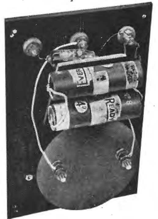
Interior view showing the valve and batteries.
